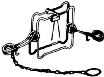
*Figure 2. Conibear with trigger spread*
